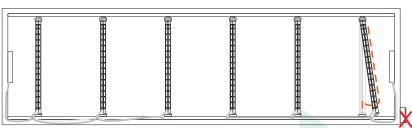
**Step Four:** install each of the LEDrofit lamps into the sockets by inserting one end in the "spring socket" then compressing the spring enough to swing the opposite end over and into the fixed socket.
