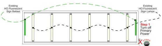
Step One: turn off primary power (main power to the sign's branch circuit).
