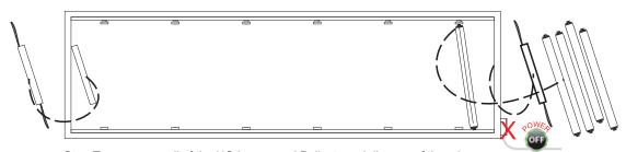
**Step Two:** remove all of the HO Lamps and Ballasts and dispose of them in accordance to local regulations. In this step, cut all ballast leads and remove them from the sockets, or tuck the leads under the raceways.
