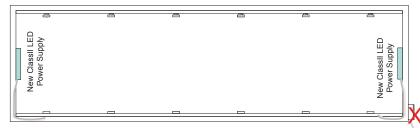
**Step Three:** mechanically fasten the New Allanson ClassII LED Power Supply and with the primary power still off, connect the primary wire(s) to the existing primary circuit.
